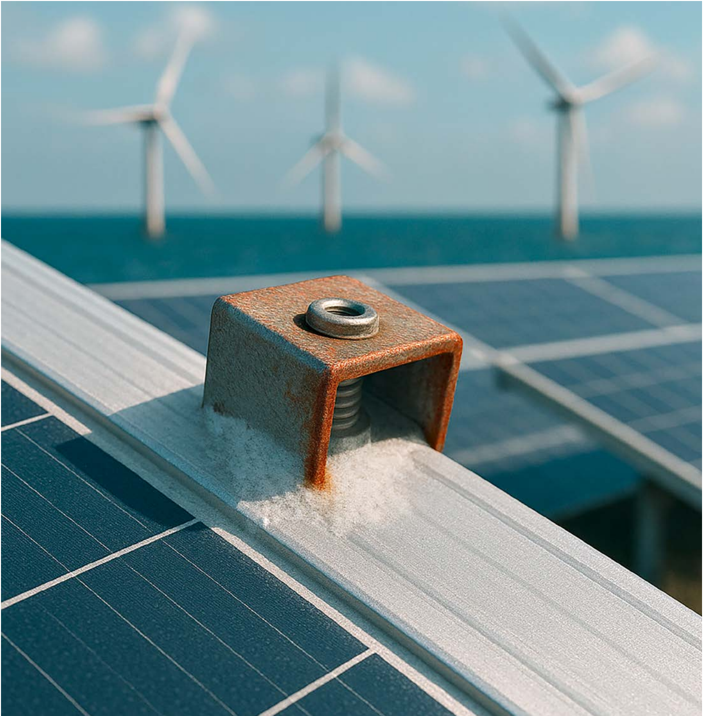
Corrosion at the material contact between steel and aluminum.
