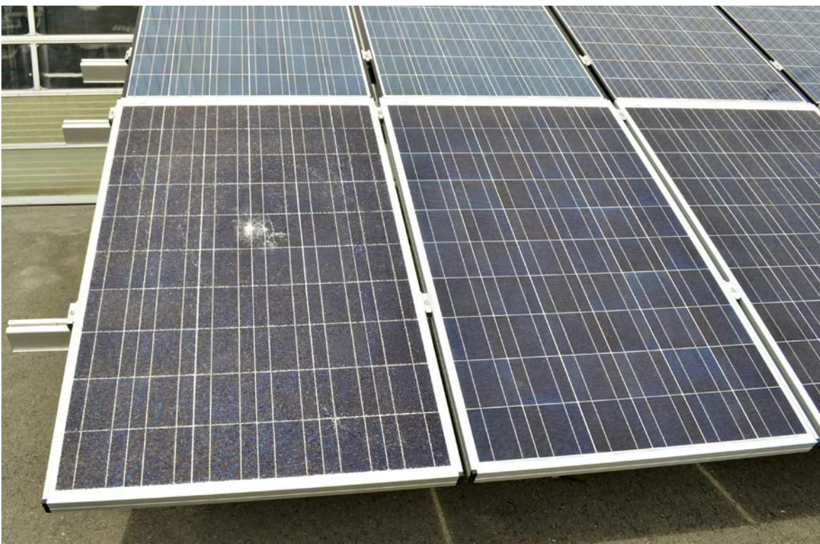
Glass breakage due to hail: This module should be replaced.
