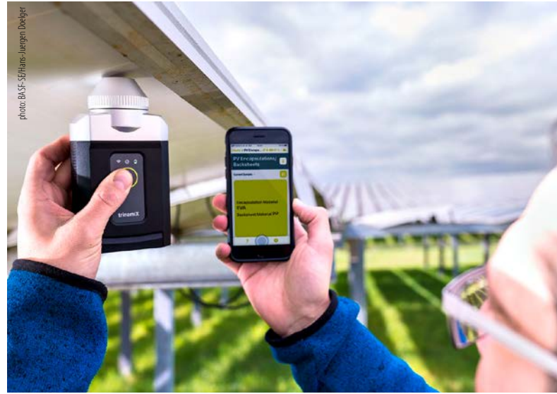
The new test device from Trinamix makes it easy to check the back sheets in the solar field.
