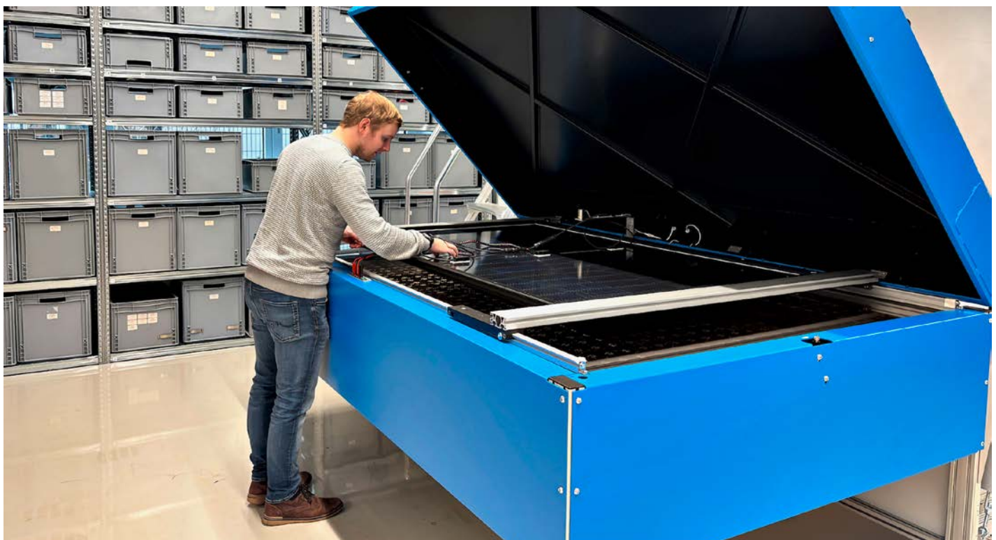
The MBJ Sunlike Lab is a solar simulator with built-in electroluminescence measurement for PV modules.
