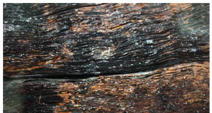
Burnt lithium cell of a solar storage device.
